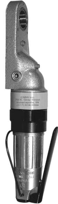
Light weight and rugged construction, this CMW Pneumatic Power Handle requires a clearance of only 1-1/2" with a standard ring and 2" with an extended ring. In most situations this allows dressing of electrodes without removal from the welder. Operating at a cutting speed of 1200 rpm, it enables the operator to dress electrodes quickly and accurately. Cutters and guide rings are easily replaced. These must be matched to the electrode nose and are selected from the chart below.
