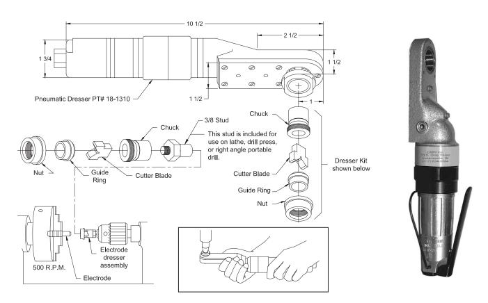
Light weight and rugged construction, this CMW Pneumatic Power Handle requires a clearance of only 1-1/2" with a standard ring and 2" with an extended ring. In most situations this allows dressing of electrodes without removal from the welder. Operating at a cutting speed of 1200 rpm, it enables the operator to dress electrodes quickly and accurately. Cutters and guide rings are easily replaced. These must be matched to the electrode nose and are selected from the chart below.
