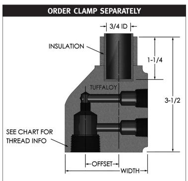
To determine distance adapter sticks out from holder, deduct 1/2-in. from length of adapter selected. Water tubes 1/2-in. longer than adapter will install approximately flush with adapter face.
