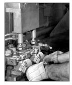
A Case Study: Joining a piece of metal to itself is always tough. This job was done with an Equa-Press holder - two at a time. Lower clamp faces, carrying current, contact parts near the weld areas to avoid current bypassing weld projections. Two standard swivel tips make four welds, two per part.
