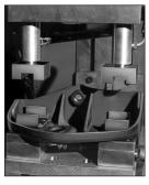
A Case Study: Projection welding brackets to automotive frame assemblies is twice as fast with an Equa-Press dual tip holder. Lower welding fixture acts as an inspection device, so warped parts are discovered before welding. Inspection time and scrap loss are both reduced.
